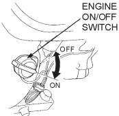
Figure 10. Engine ON/Off Switch
